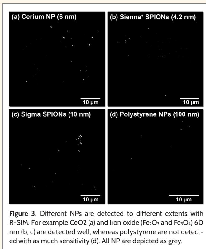
**Figure 3.** Different NPs are detected to different extents with R-SIM. For example CeO<sub>2</sub> (a) and iron oxide (Fe<sub>2</sub>O<sub>3</sub> and Fe<sub>3</sub>O<sub>4</sub>) 60 nm (b, c) are detected well, whereas polystyrene are not detected with as much sensitivity (d). All NP are depicted as grey.
