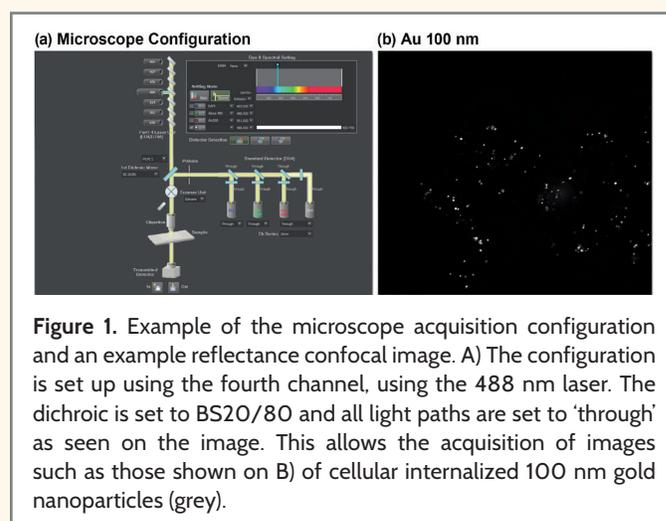
**Figure 1.** Example of the microscope acquisition configuration and an example reflectance confocal image. A) The configuration is set up using the fourth channel, using the 488 nm laser. The dichroic is set to BS20/80 and all light paths are set to 'through' as seen on the image. This allows the acquisition of images such as those shown on B) of cellular internalized 100 nm gold nanoparticles (grey).
