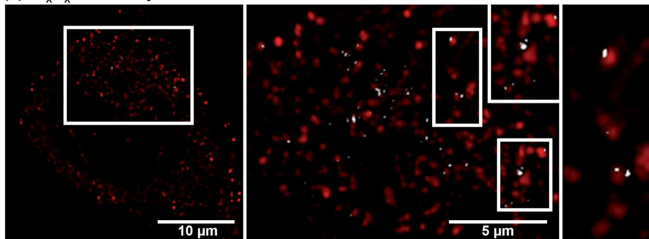
**Figure 4.** RCM and R-SIM of SPIONs (Fe<sub>2</sub>O<sub>3</sub> and Fe<sub>3</sub>O<sub>4</sub>) 60 nm. NP signal in grey and lysosome signal in red. R-SIM leads to a substantial increase in resolution when compared to RCM for performing colocalization studies.
