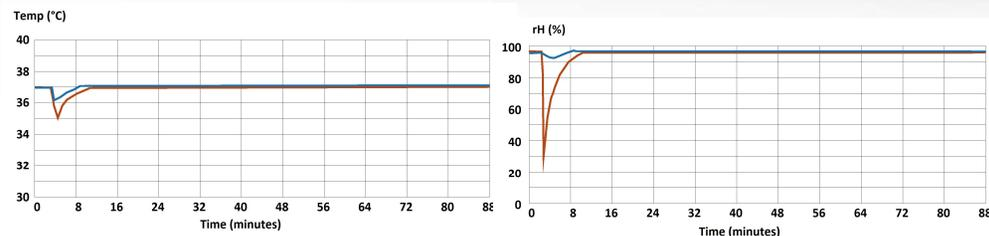
(Above) Temperature and humidity plots over time after front door (red) or side door (blue) were opened. In these examples, the side door was not enclosed in a microscope enclosure / incubator. With our included microscope enclosure, even more temperature and humidity stability is maintained between the microscope stage and the incubator.
