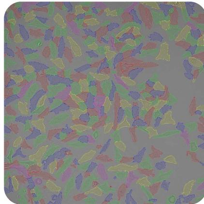
Acquisition of a transmitted light image without contrast (no phase contrast or DIC) can now be used to compute a **Volume Contrast** enhanced result image in which the volumetric shape of objects produces contrast. The contrast image can be used for segmentation.
