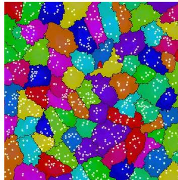
The spot counting tool detects and counts granularity in cells, creating boundaries between cells and reporting number of granules per cell.
