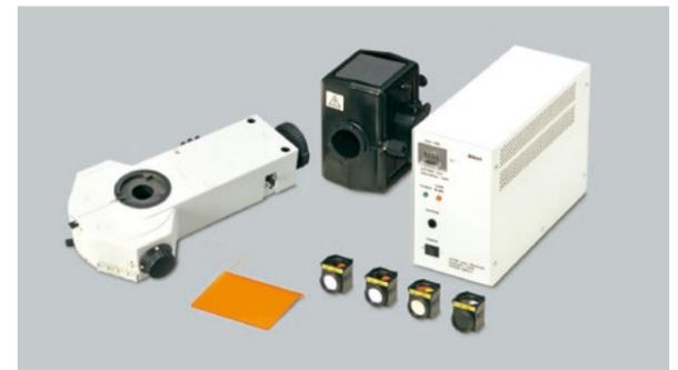
CI-FL Epi-Fluorescence Attachment with mercury lamphouse and power supply
