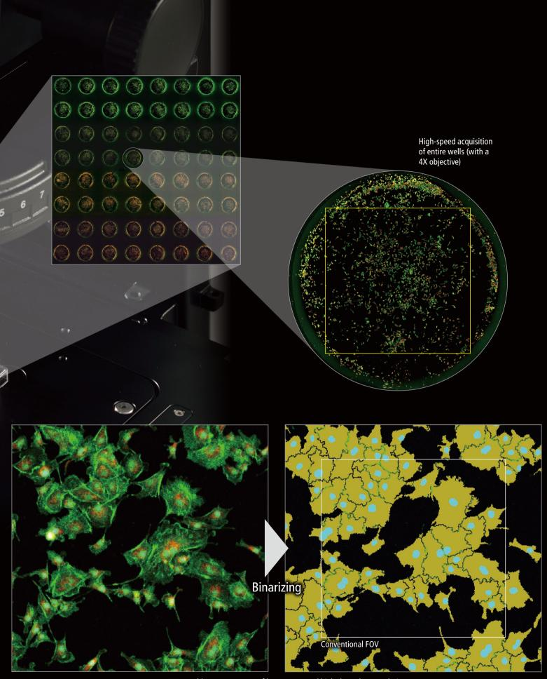
Large FOV enables measurement of larger areas and high-throughput analysis.
