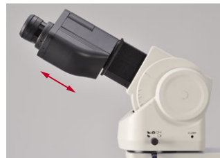
Eyepiece length can be extended by up to 40 mm.
