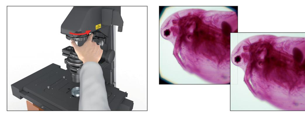
Open the Field Diaphragm – Once open, the edges should extend just past the desired field of view. Fine centration of field diaphragm may be performed while mostly (but not fully) opened.
