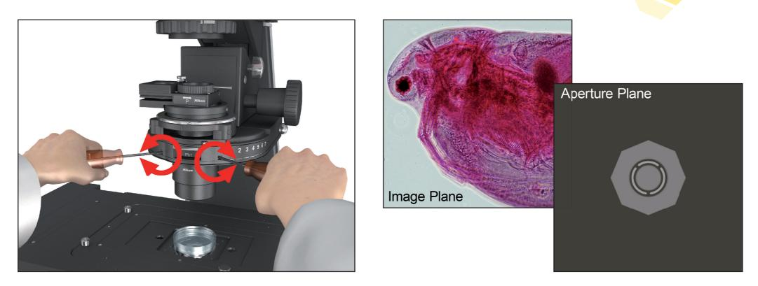
**OPTIONAL: Center Phase Annulus** – Insert a pair of 2 mm hex keys into the illustrated slots and rotate to center the image of the condenser phase annulus (light gray ring) within the image of the fixed-position phase annulus etched into the objective (black ring). The Bertrand lens may now be removed and the system is ready for phase contrast imaging.
