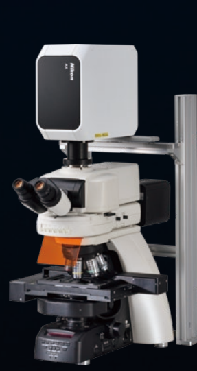
Configuration with Ni-E focusing stage type
